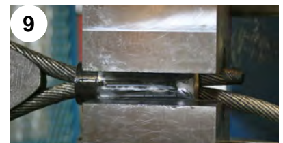
9 If a second swaging is required, open dies and swage the second part of the ferrule. Close dies.
