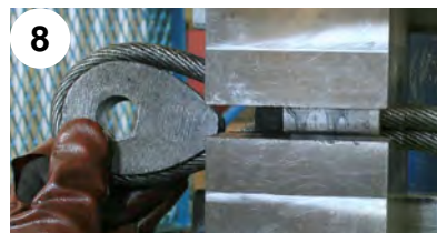
8 Swage T-LOC and ferrule (or first part of the ferrule, if the assembly is too long for the dies). Close dies.
