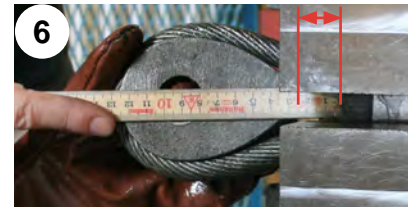
6 Measure. Distance T-LOC and solid thimble before swaging must be at least 2 times the nominal diameter. For pointed thimbles the distance can be reduced.
