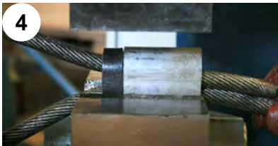
4 Mount in lubricated dies. T-LOC must be positioned next to T ferrule.
