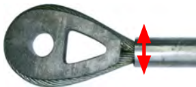
Splitting risk on 2160 grade wire rope without T-LOC
