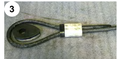
3 Incorporate thimble, if used. Further adjustment while swaging.
